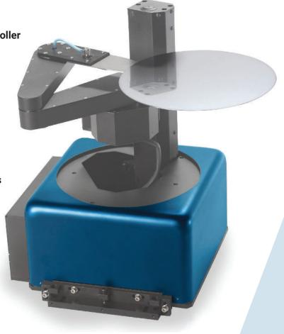
Hine atmospheric robots are high-performance substrate handling solutions for semiconductor applications. These SCARA type robots provide reliable and clean transfer mechanism for atmospheric front ends. Hine atmospheric robots transfer a wide variety of substrates including SEMI standard wafers, reticles and masks.
