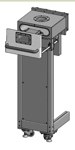
Designed to provide cassette loading and unloading capabilities for the Constellation family of cluster systems our Vacuum Cassette to Cassette Load Ports (CLP) can be customized to adapt to a customer's specific requirements. The various Load Port configurations are built around the Hine Automation Vacuum Elevators with material indexing and positional sensing capabilities.
